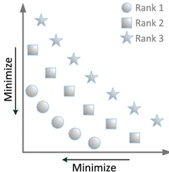
Figure 5-4 Non-dominated sorting for a multi-objective function [132]
