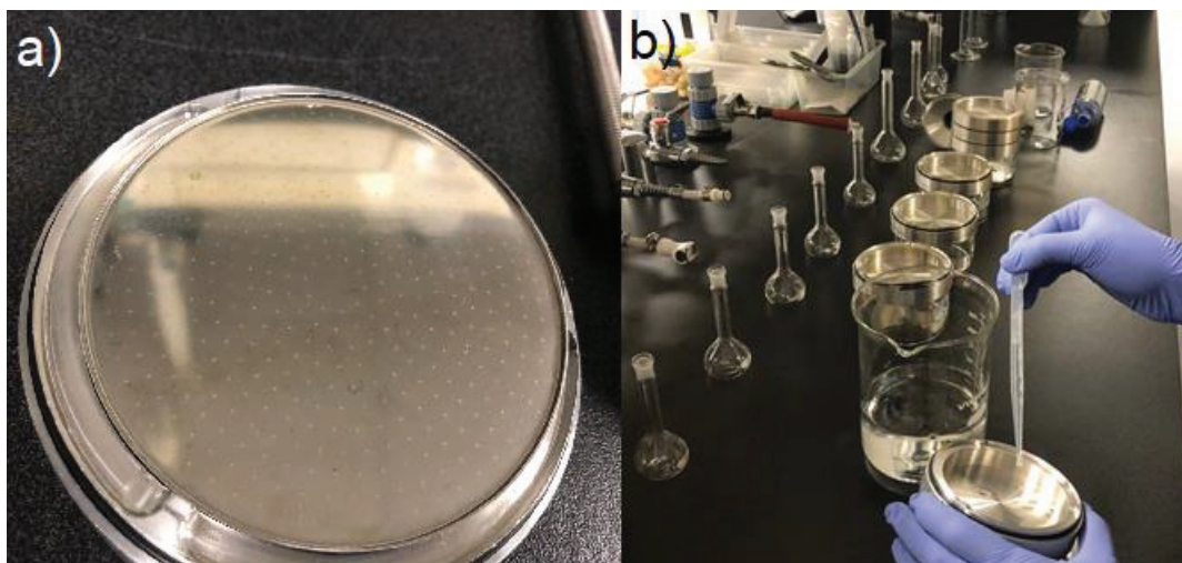
Figure 4-4 a) Deposited drug in cascade impactor plate b) washing cascade impactor stage
