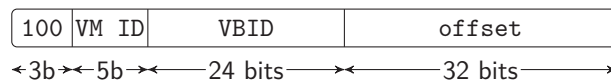
Figure 3.5: Partitioning the VBI address space among virtual machines, using the 4 GB size class (100) as an example.
