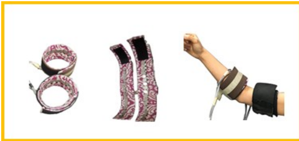
Figure 2.5. Custom-made Force myography bands. Reproduced from [56] with permission.
