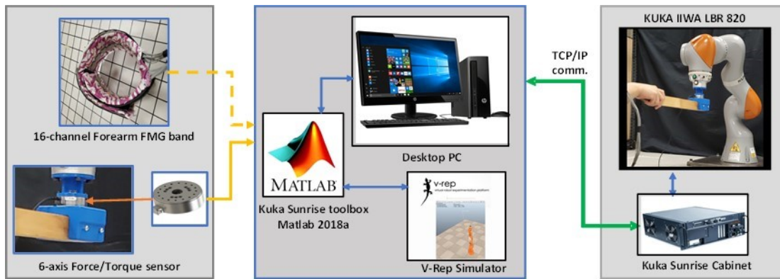
Figure 2.10. Force control implementing compliant collaboration with the Kuka robot via external interactive applied force.
