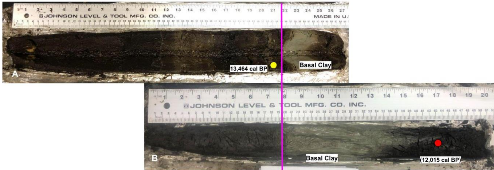
Figure B.6. Cores 5 and 6 showing interpreted re-core of Drive 6.
