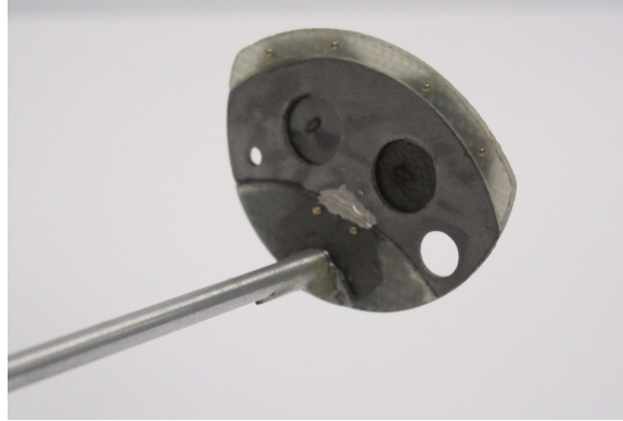
Figure 3.5: Photograph of the target mounted on the left position of the target wheel, taken after the experiment. Mounted on the right position of the target wheel was a fluorescent screen for visual checks of the beam profile. The photograph was reprinted from private communication with Phil Voss.
