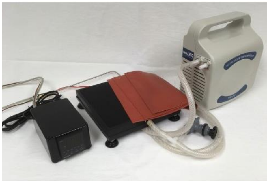
Figure 2-1 Vacuum hot plate (Welch™) used for hand spraying anodic catalyst layers; from left to right, components are digital temperature controller, vacuum hot table, three sheets of silicone rubber and vacuum pump.
