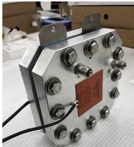
Figure 2-4 Pictures of cell assembly process of FuelCellStore water electrolyzer with a sprayed MEA. Components that need to be assembled from outside to inside are the anodic end plate, outer gasket, flow field embedded current collector, anodic Ti PTL, inner gasket and sprayed. Reversing the steps from 1 to 5 is the process for assembling cathodic components.
