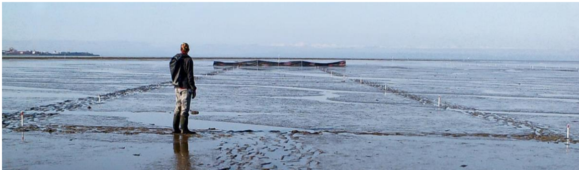
Figure 3.3. Treatment transect with the obstruction tarp installed 120 m from shore. White, 15 cm tall, stakes mark the corners of each 10 m x 10 m plot.
