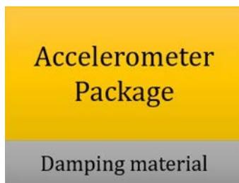
Figure B.3 The proposed mechanical low pass filter for
