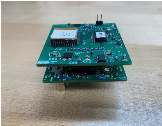
Figure 5.3 Double layer PCB board for testing
