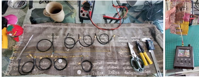
Figure 6.12. Henry's set up to test the antennas, including clippers, a multimeter, and coaxial cables, which needed to be attached to each sample, and testing an antenna sample with a vector antenna analyzer.
