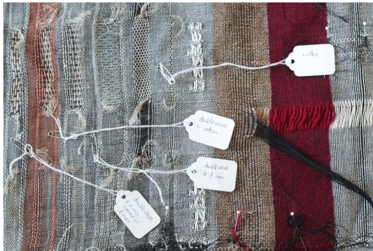
Figure 6.11. A photograph of the labelled antenna sample before cutting and scanning (the observant reader may recognize some pins and knots from Figure 6.8).
