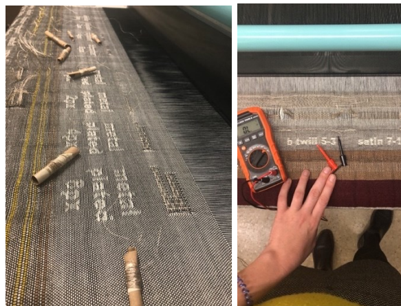
Figure 6.9. Weaving with the conductive material on separate bobbins as additional weft, and measuring connectivity with the multimeter.
