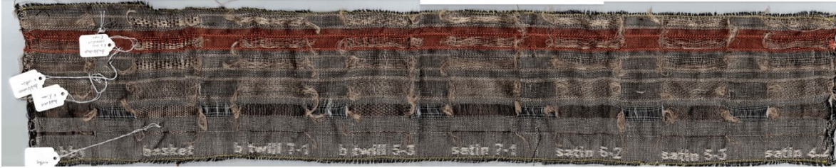
Figure 6.10. A scan (stitched together in Photoshop) of a woven antenna sample, with labels and woven text indicating the difference between swatches.
