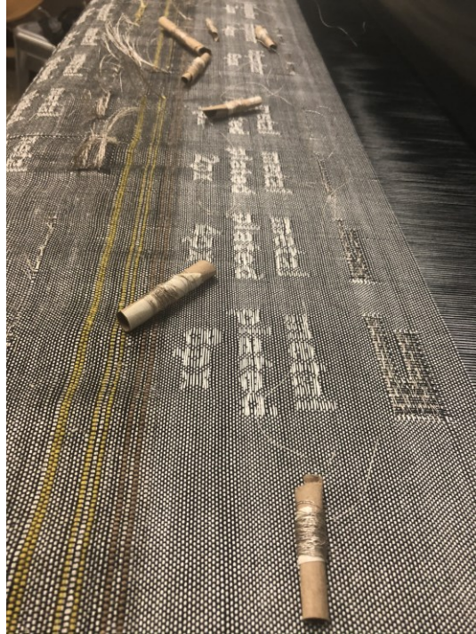
Figure 3.7. First explorations of the Woven Wi-Fi antenna on the TC2 loom at the Unstable Design Lab.
