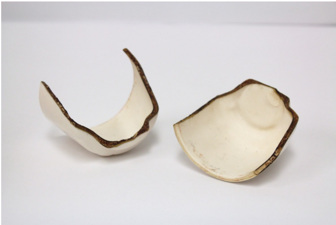
Figure 5.15. The outer part of the kintsugi repaired cup broke again during the assembly process.
