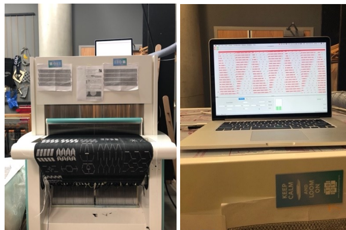
Figure 6.4. The loom with some first weaving samples, and the MacBook pro with the TC2 software.
