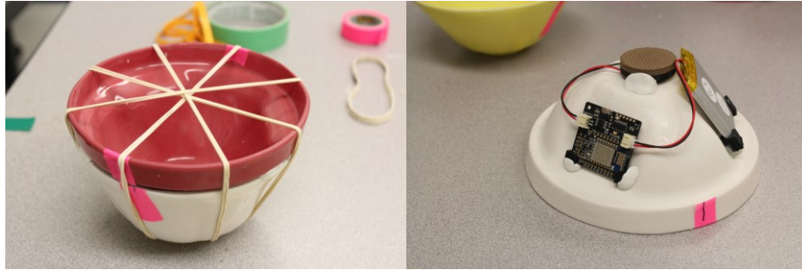
Figure 5.13. Two assembly steps of the Morse Things: the housing of the electronics, and the applied elastic bands to keep pressure on the transducer as the sugru dries.
