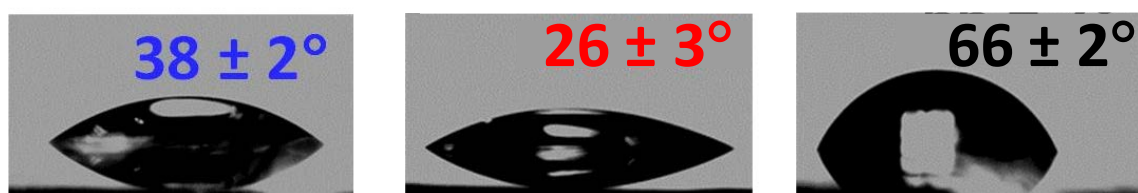
Figure 4.2 Water contact angle measurements on the N3C11S-Au before (left) and after the tethering of \equiv\text{-O-CB}[7] via CuAAC (middle), and upon the subsequent incubation in 50\ \mu\text{M} FcMeOH for 1 h. The volume of the water droplet for each measurement was kept at 1.5\ \mu\text{l} . The standard deviations were based on 3 randomly selected spots on three independently prepared gold samples.
