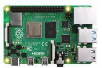
Figure 2.2: Raspberry Pi 4 Model B [11]
