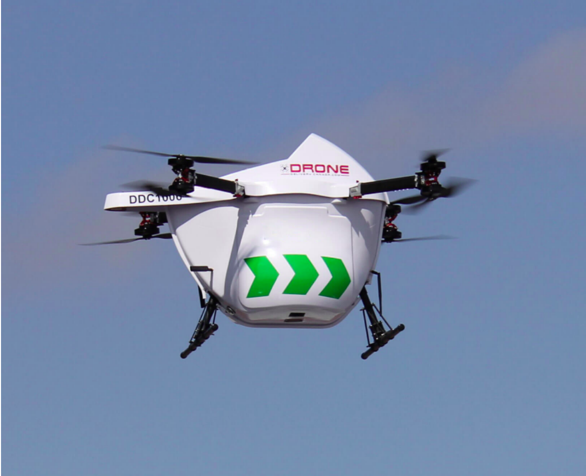
Figure 2.1: Sparrow, a GPS-based autonomous navigated drone introduced by Drone Delivery Canada [3]
