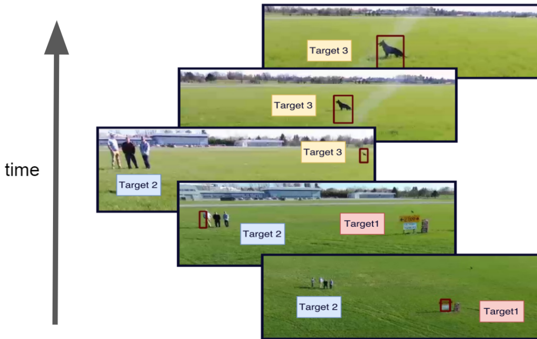
Figure 2.5: Real environment test: taking a close-up image of the 30*30cm object by flying 150m and only three clicks on the user interface [38].
