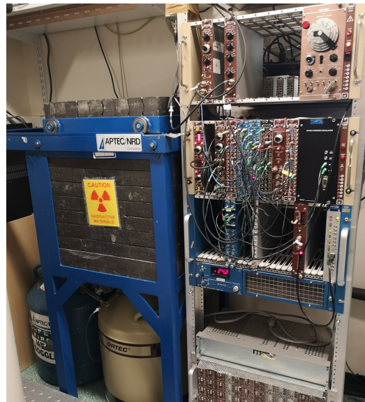
Figure 3.1: (Left) The interior of the shielding of the GEARS detector is shown, with a Cd/Cu cylinder surrounding an Al can, which encases the detection crystal. [7]. (Right) The lead shielding around the GEARS detector is pictured next to the DAQ system.
