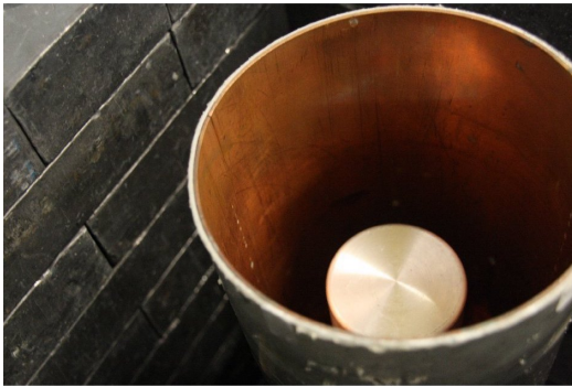
Figure 3.1: (Left) The interior of the shielding of the GEARS detector is shown, with a Cd/Cu cylinder surrounding an Al can, which encases the detection crystal. [7]. (Right) The lead shielding around the GEARS detector is pictured next to the DAQ system.
