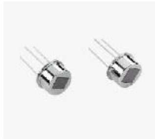
Figure 18: Murata IRA-E410QW1 Pyroelectric Sensor
