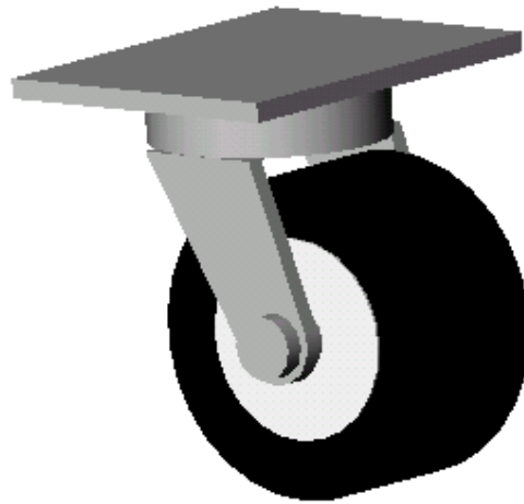
Figure 4: 3-D View of a 2" Diameter Swivel Caster
