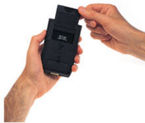
Figure 2. Rear View of Handspring Visor, showing Springboard Expansion Slot and Card (Handspring 2001a)
