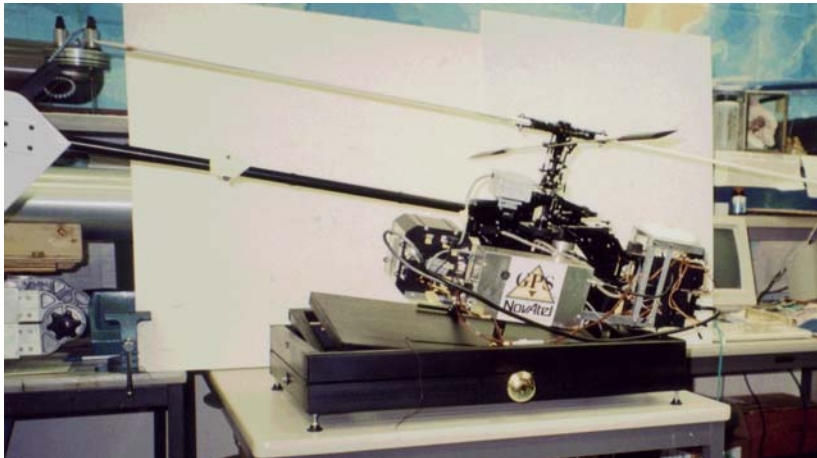
Figure 6: Multi-plane Testing Table in a Forward Roll Tilt Configuration
