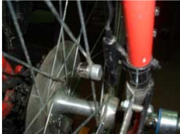
Figure 4: Speed Sensor Mounted on the Ranger
