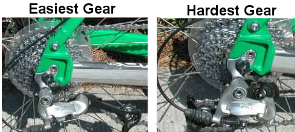
Figure 7.1: Standard rear derailleur. (courtesy HowStuffWorks.com)
