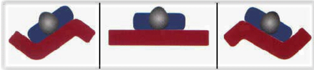
Figure 1: Turning Motion of the Freedom Bed ( www.pro-bed.com )
