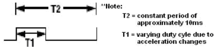
Figure 15: ADXL202 output pulse
