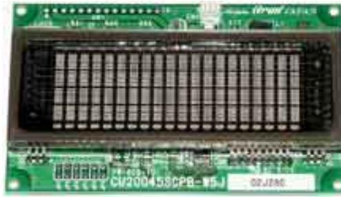
Figure 4-8: Picture of G-7002 VFD
