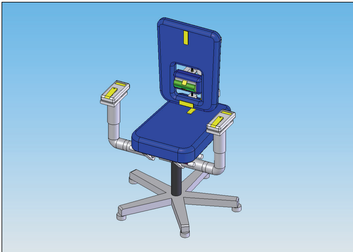
Figure 3: Sensors on the ACE Chair. Sensors are highlighted in yellow.
