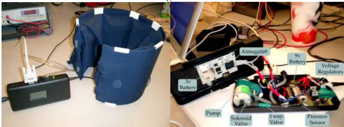
Figure 2.2 – EMS Proof-of-Concept enclosure and control unit
