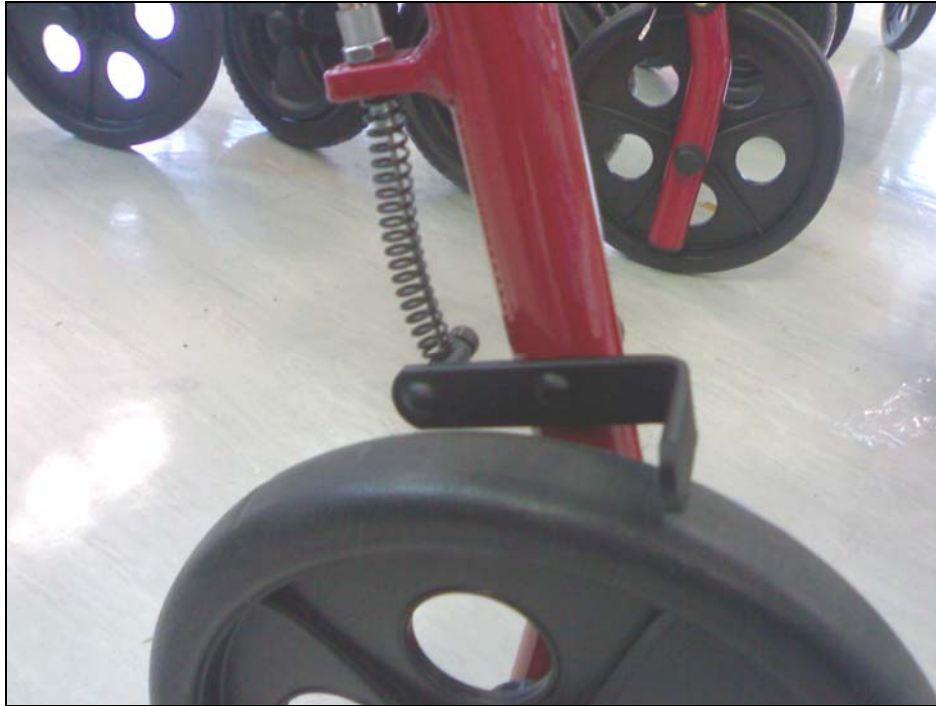
Figure 3: Walker brake type 1
