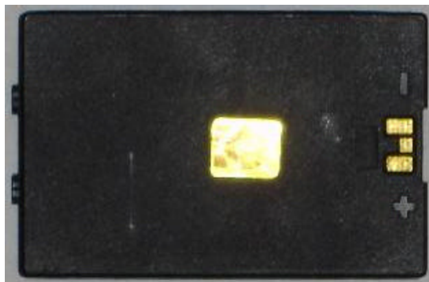
Figure 8: Battery Mock Up (height = 2in and length =2.65in)
