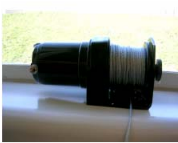
Figure 7: Electric winch for cabling subsystem
