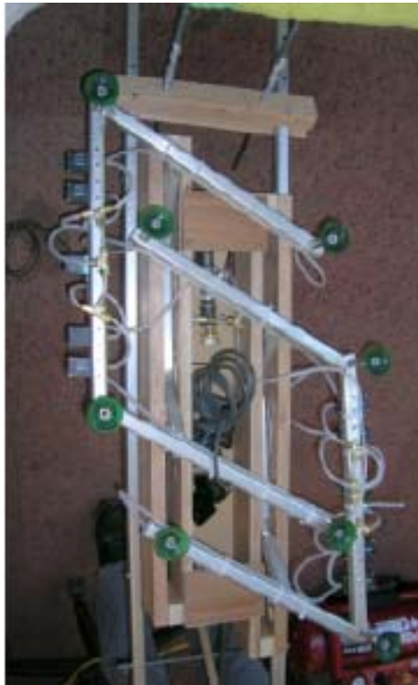
Figure 6: Aluminum legs and wooden paths of the down-climb subsystem
