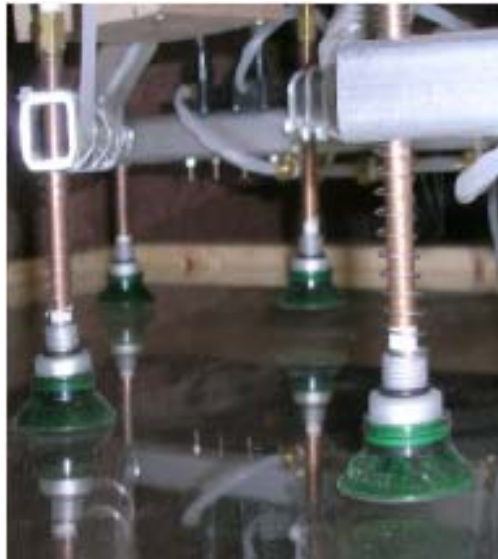
Figure 4: Suction cups with level compensators
