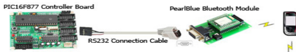
Figure 24: The Pearl Blue Bluetooth module connection diagram
