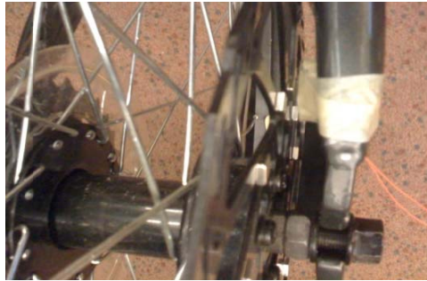
Figure 3 Speed Sensor Placement
