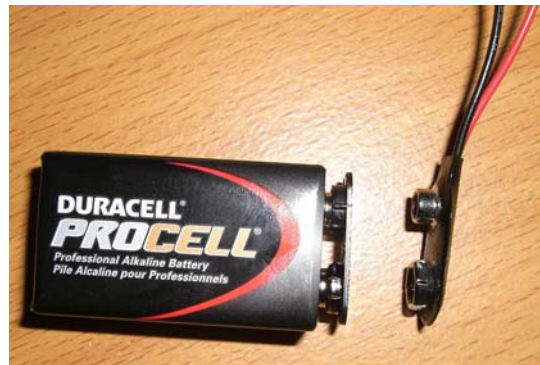
Figure 16. a 9V Battery to power the system
