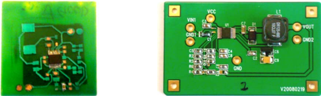
Figure 4-3: “In-house” Board and 3 rd -Party Fabricated Board
