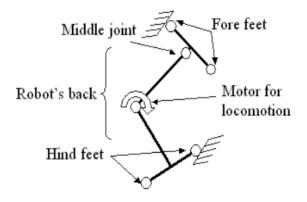
Figure 5: Proposed Operation of a simple geckoinspired climber [6]
