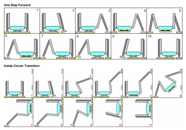
Figure 8: Step by Step Operation of Mattoid
