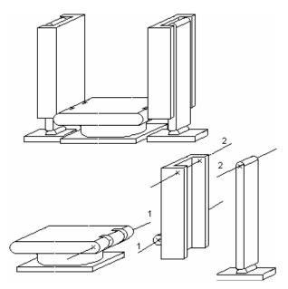
Figure 7: Sketch of the proposed crawler design concept
