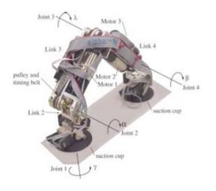
Figure 2. The Under Actuated Climber, University of Utah [3] This simple robot design can be used to transition between flat surfaces at any arbitrary angle, which suggests that there are aspects of this design to be researched further.
