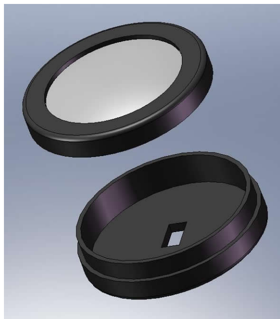
Figure 22: Exploded View of PTT Enclosure
