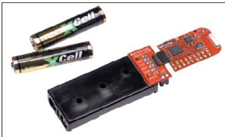
Figure 15: ez430-RF2500T Target Board with Battery Board [4]
