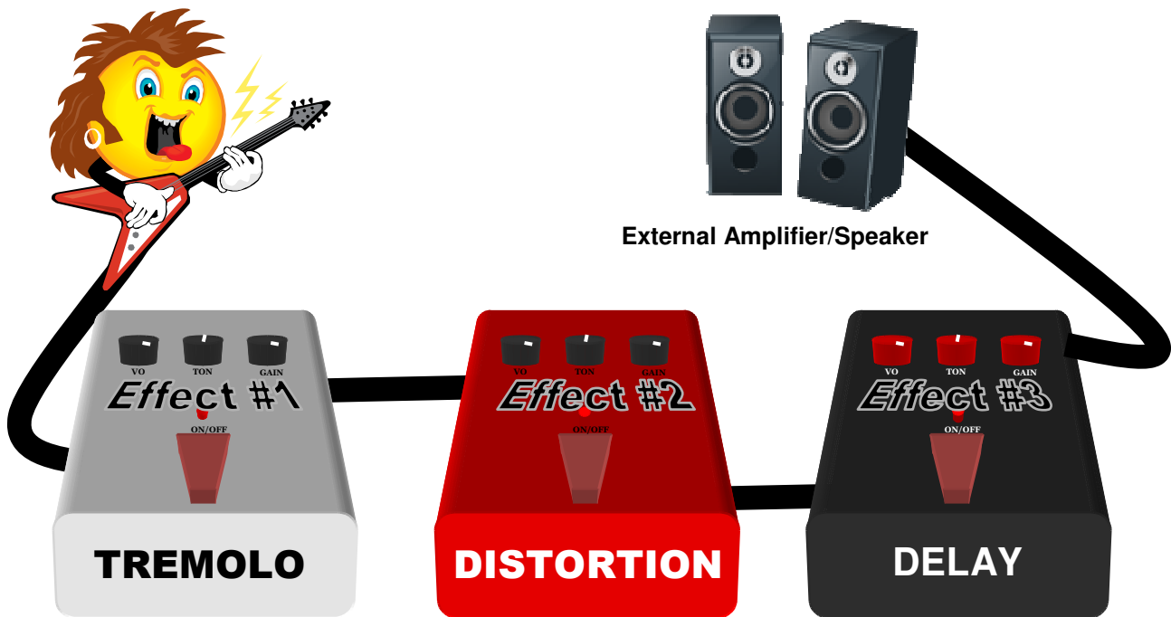
Figure 1: Diagram of Guitar-FX Processing
