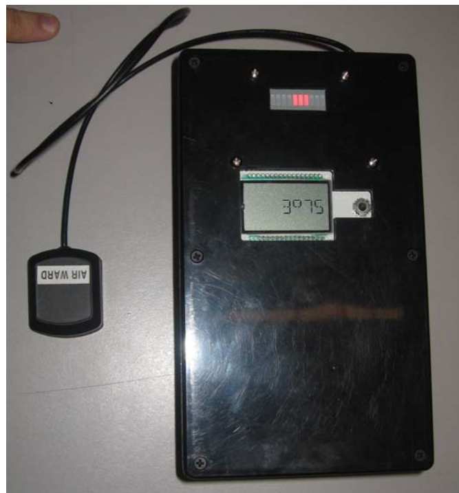
Figure 6: A lean angle displayed and visually through LED bar (note degree is a decimal place)
