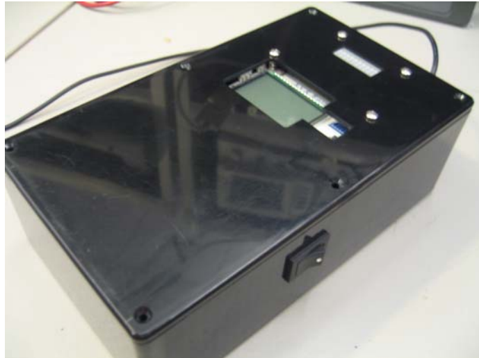
Figure 5: Power switch located at side, windows on lid for LED bar and LCD screen
