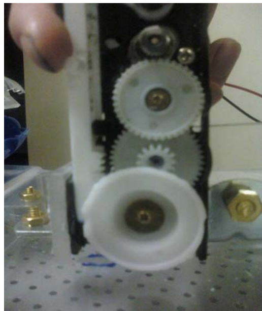
Figure 4: DC motor drives the gear network and linear motion moves the actuation enclosure vertically
