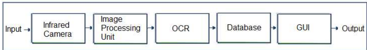
Figure 2: High Level Overview of the APE System.
