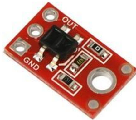
Figure 11. Picture of Wheel Speed Sensor
