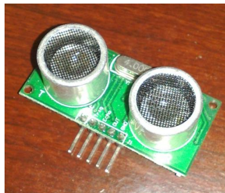
Figure 10. Picture of Ultrasonic Distance Sensor
