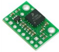
Figure 13. Picture of Accelerometer Module
