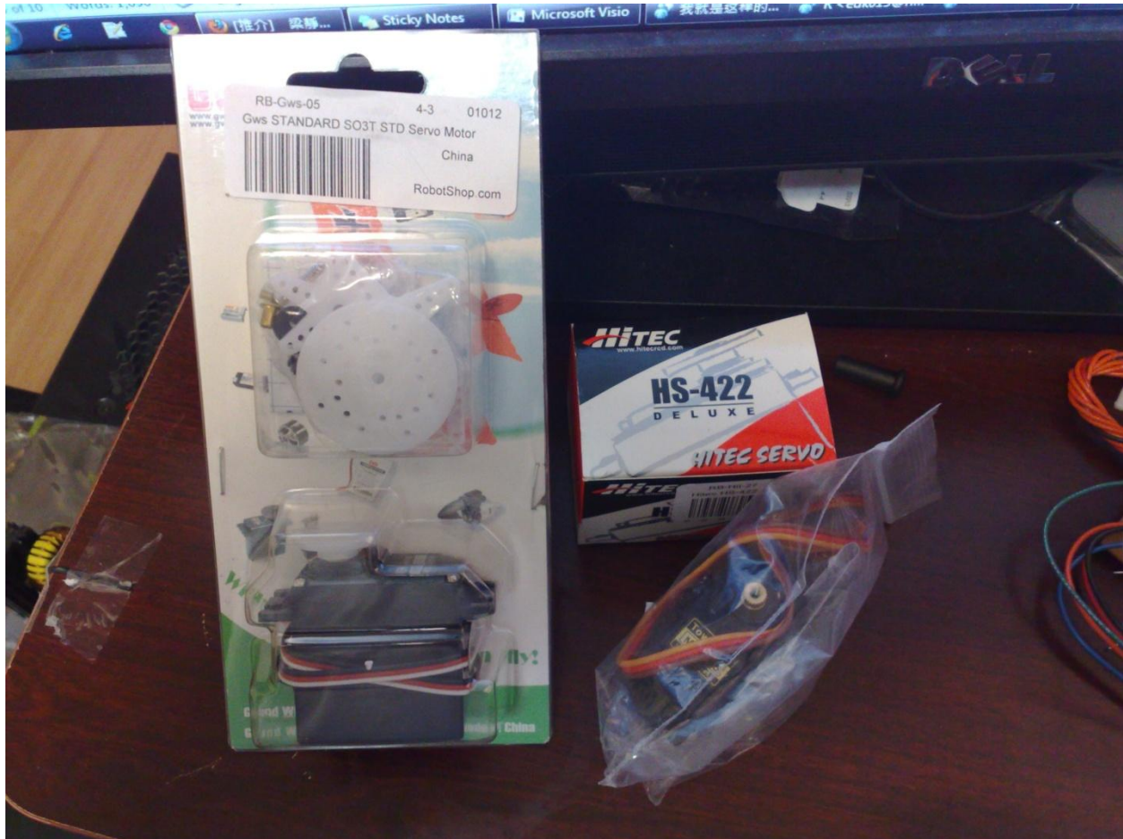
Figure 22. Servo Motors used by the Robotic Arm
