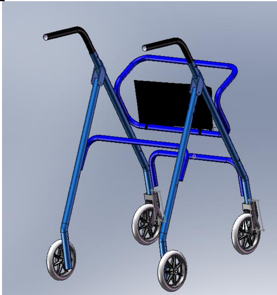
Figure 11 - Rollator frame rear bar modification
