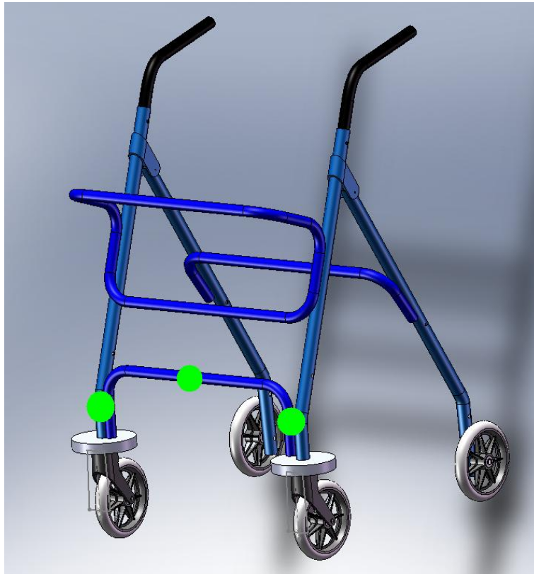
Figure 13 – Placement of the LEDs on the rollator
