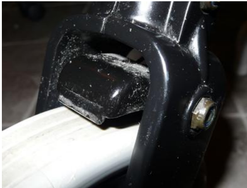
Figure 8 - Rollator integrated manual wheel lock (alternate view)
