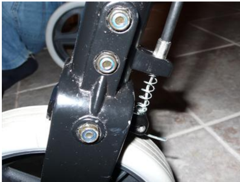
Figure 7 - Rollator integrated manual wheel lock
