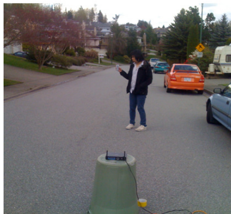
Figure 4: Test setup to find the WiFi range of DT.
