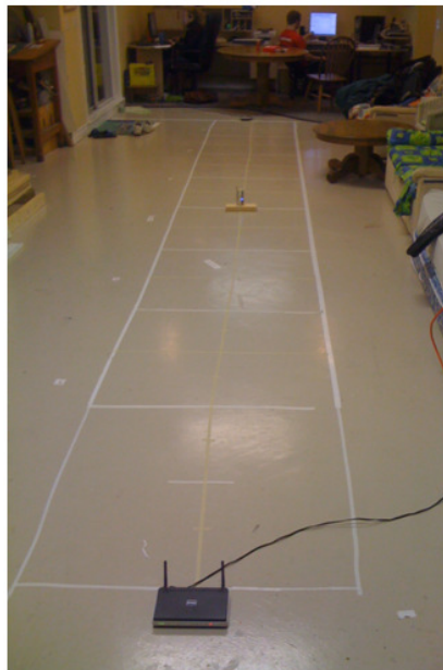
Figure 6: Test setup for signal strength attenuation, Gumstix middle, access points on either end.
