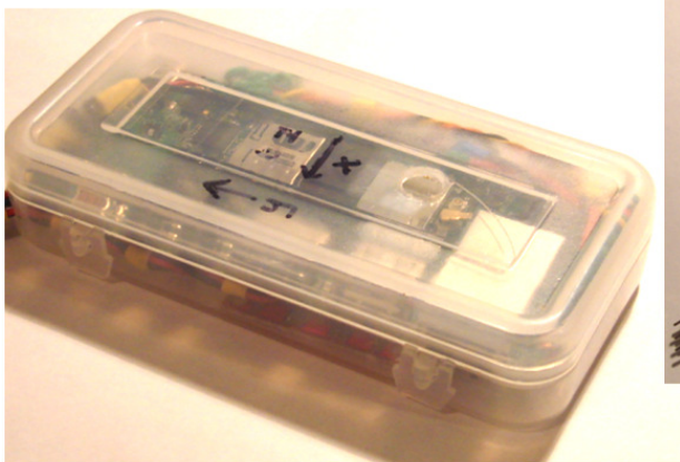
Figure 2: The assembled module for the PosiTrack system.
