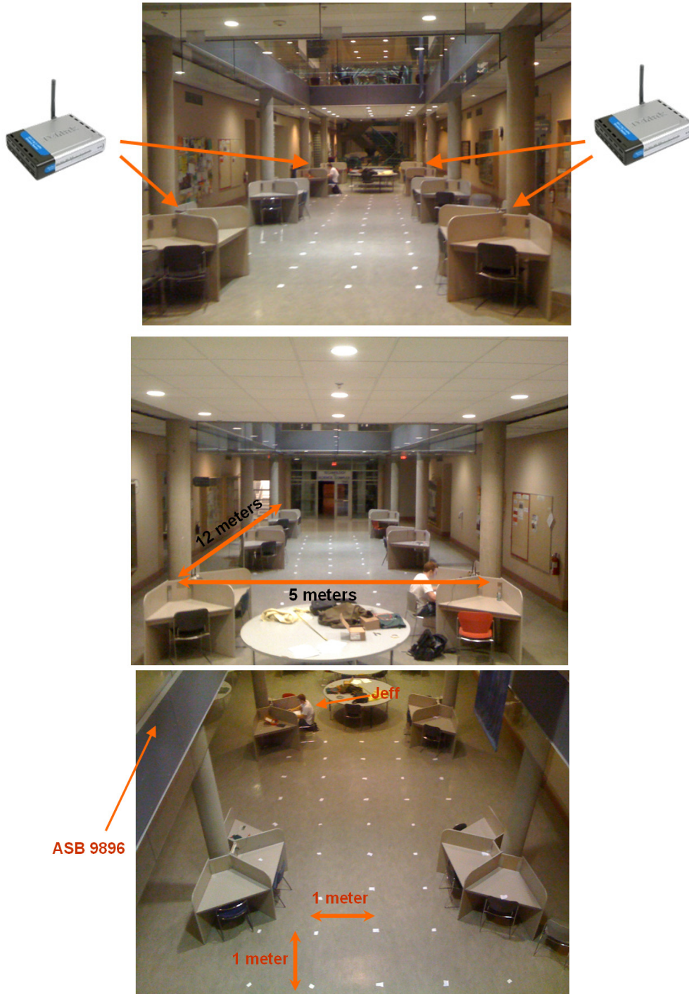
Figure 16: Signal strength mapping of 4 access points in a 5m x 12m area in a 1m x 1m grid.
