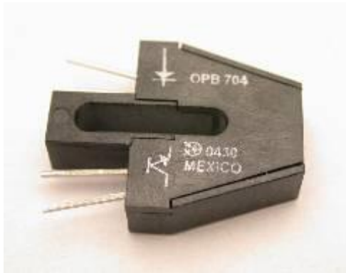
Figure 14: Active Bag OPB704 IR Sensor. [7]
