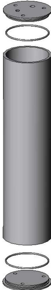
Figure 2: Perspective view of the final enclosure design (exploded view)
