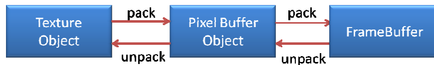
Figure 4.7: OpenGL Texture to Framebuffer Mapping [7]
