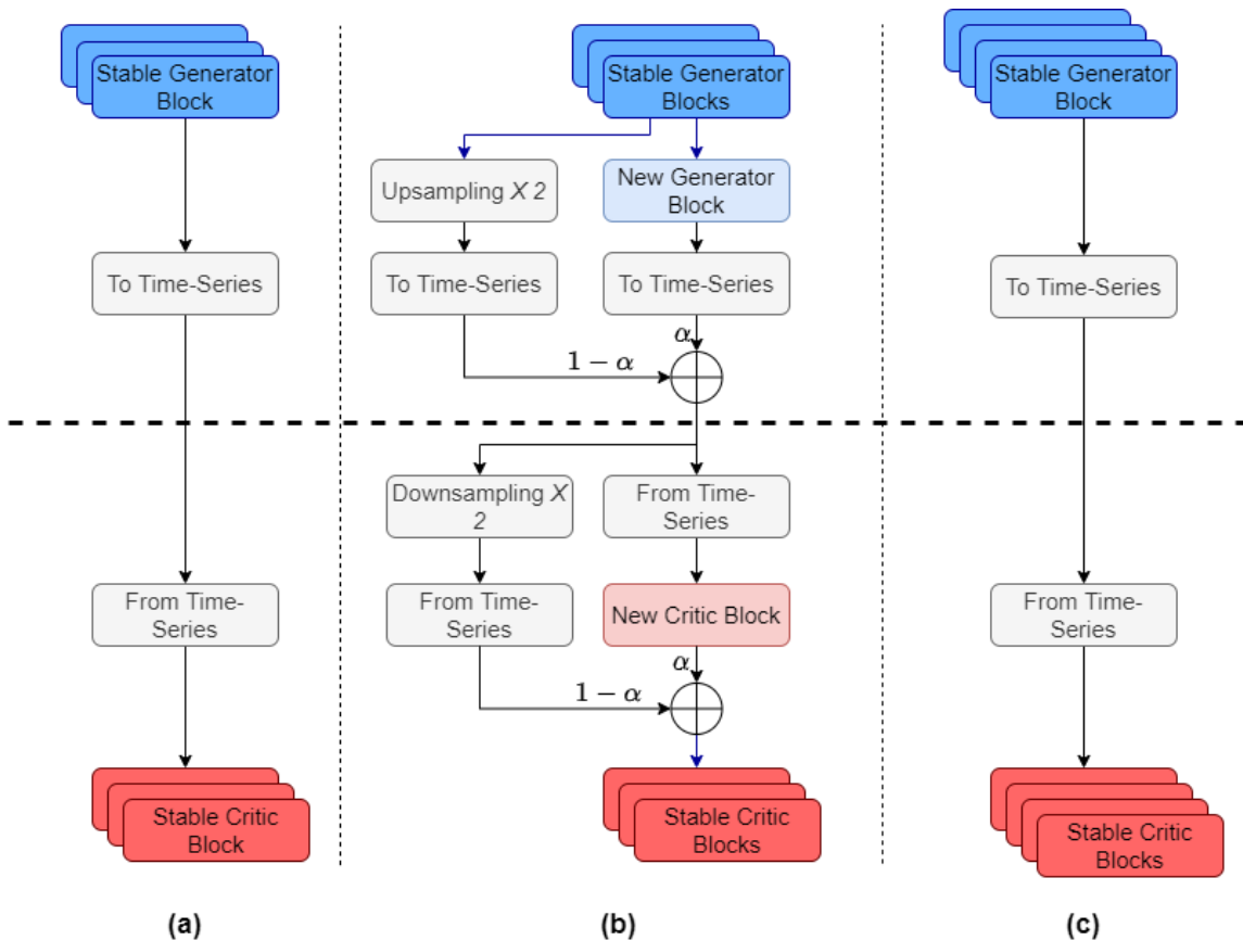
Figure 4.1: The fading procedure proposed by [34] as adapted for one time-series data in [117] and PowerGAN. In (a) we see the currently stable generator and critic during an intermediate stage of training; note that generator (critic) contains a upsampling (downsampling) step. The blocks “To Time-Series” and “From Time-Series” are implemented via 1D convolution. In (b) we see the fading stage. On the generator side, the output of new blocks is slowly faded in, using a linearly growing parameter \alpha , with an nearest neighbor upsampling of the output of the stable blocks. Similarly, on the critic side, the features created by the new block are slowly merged in with previous inputs to the existing critic blocks. Finally, (c) shows the blocks after the fading is complete and \alpha = 1 . In PowerGAN, this fading is performed over 1000 epochs, allowing for knowledge obtained at earlier steps of training to slowly adapt as new layers are added.
