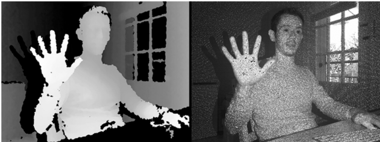
Figure 3.1.5 Depth map (left) created from light IR pattern (right) [30]
