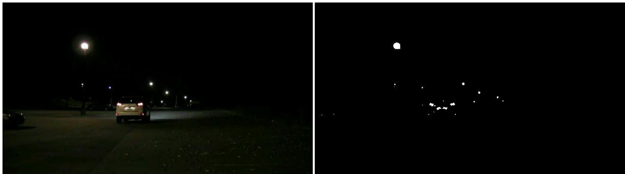
Figure 20: Original frame (left) and binary map of bright objects (right)
