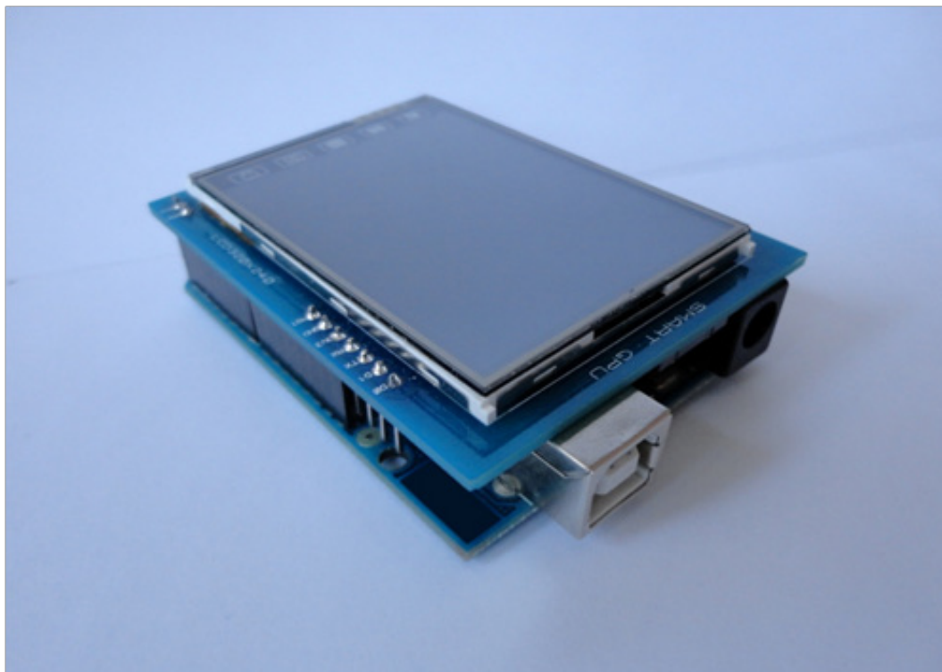
Figure 10: GPU with LCD screen mounted on an Arduino prototyping board
