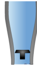
Variable Area (Float Style) for Water, DI Water, Corrosives or Compressed Air
