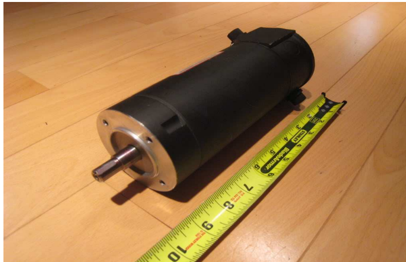
Figure 6.4 DC Power Generator
